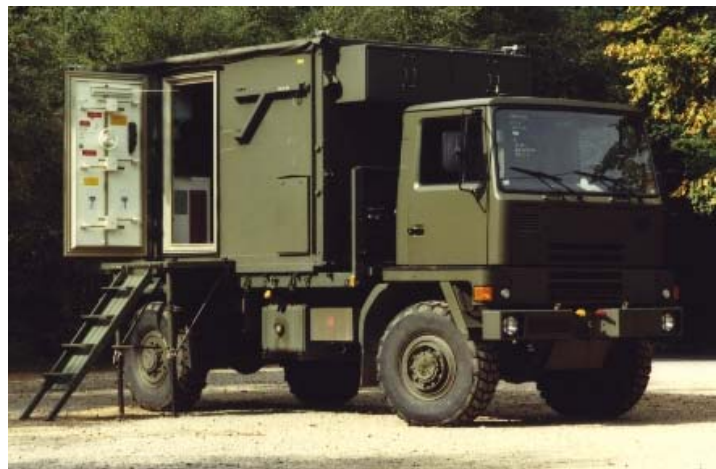
Example of General Purpose Automatic Test Equipment Vehicle used by the British Army
