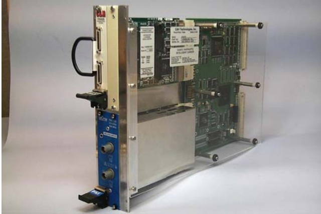
Figure 5. Example of a VXI Oscilloscope using a PXI Digitizer on an intelligent VXI to cPCI/PXI carrier
